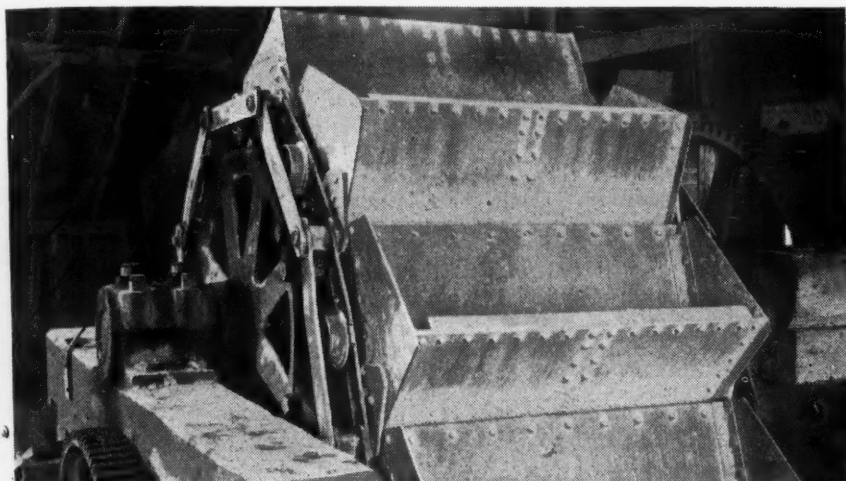
Jeffrey Heavy-Duty Bucket Elevators successfully handle Stone, Ores, Cement Clinker and similar materials in capacities up to 700 tons per hour.
